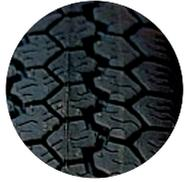
Tires must be replaced when the tread is worn down to 2/32 of an inch. Traction, particularly in bad weather, and resistance to hydroplaning is reduced as tires wear. An easy test: place a penny into a tread groove. If part of Lincoln's head is covered by the tread, you're driving with the proper amount of tread. If you can see all of his head, you should buy a new tire.
